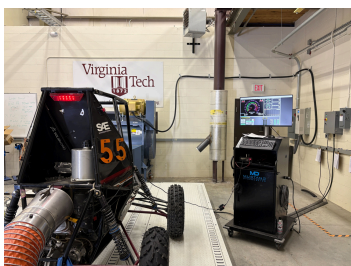
Baja SAE on the chassis dyno. Notice the exhaust control in the left photo (orange pipe at back of vehicle).
