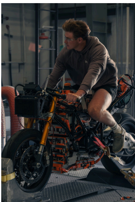
Testing BOLT VI on the Mustang chassis dyno.
