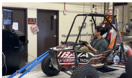
Baja SAE on the chassis dyno. Notice the exhaust control in the left photo (orange pipe at back of vehicle).
