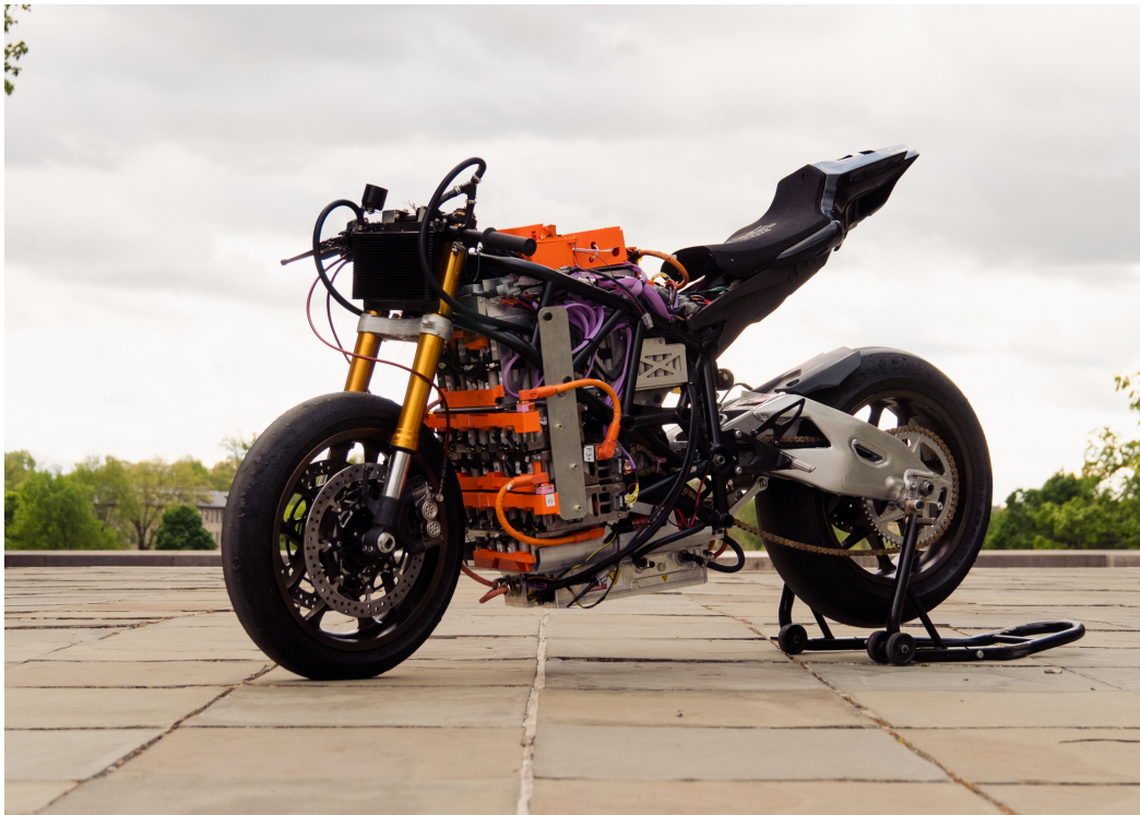
Virginia Tech's EV BOLT V with custom battery array and frame, brush-less EV motor, and student built battery management system.
