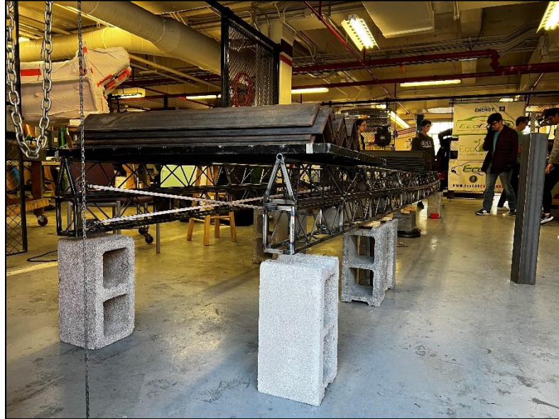
Figure 7 – This year’s steel bridge during load testing at the Ware Lab. Bridges are subjected to six load cases during competition similar to actual civil engineering structures.
